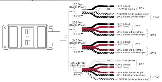
\*\* Ground wire is connected externally. Ground wire does not enter or exit the GFCI box. Although GFCI does not require Ground to operate, Ground connection is recommended and should be made at junction box.
