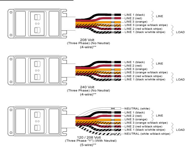
\*\* Ground wire is connected externally. Ground wire does not enter or exit the GFCI box. Although GFCI does not require Ground to operate, Ground connection is recommended and should be made at junction box.
