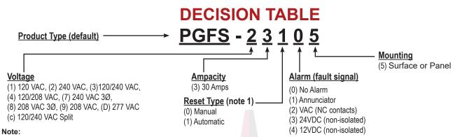
1. Manual configuration should be specified if automatic power-up, after power restoration of circuit power, could create an unsafe condition. 2. Units are configured with 18in of 10AWG, MTW / THHW / AWM, 105C, 600V, individual conductors.
